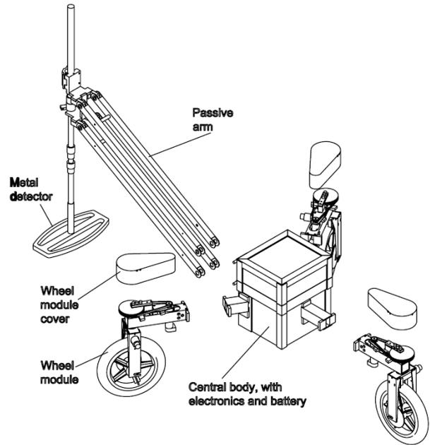
Fig. 2. Exploded view of the TriDem robot.
