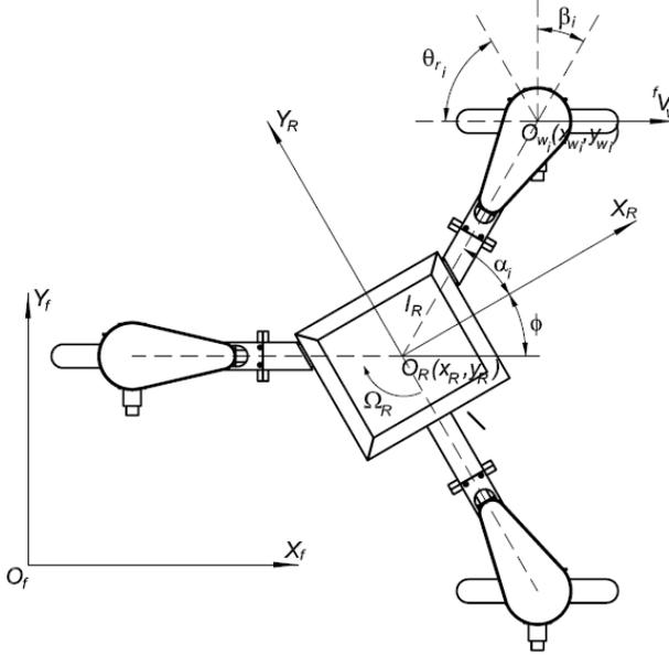
Fig. 5. Robot kinematics.
