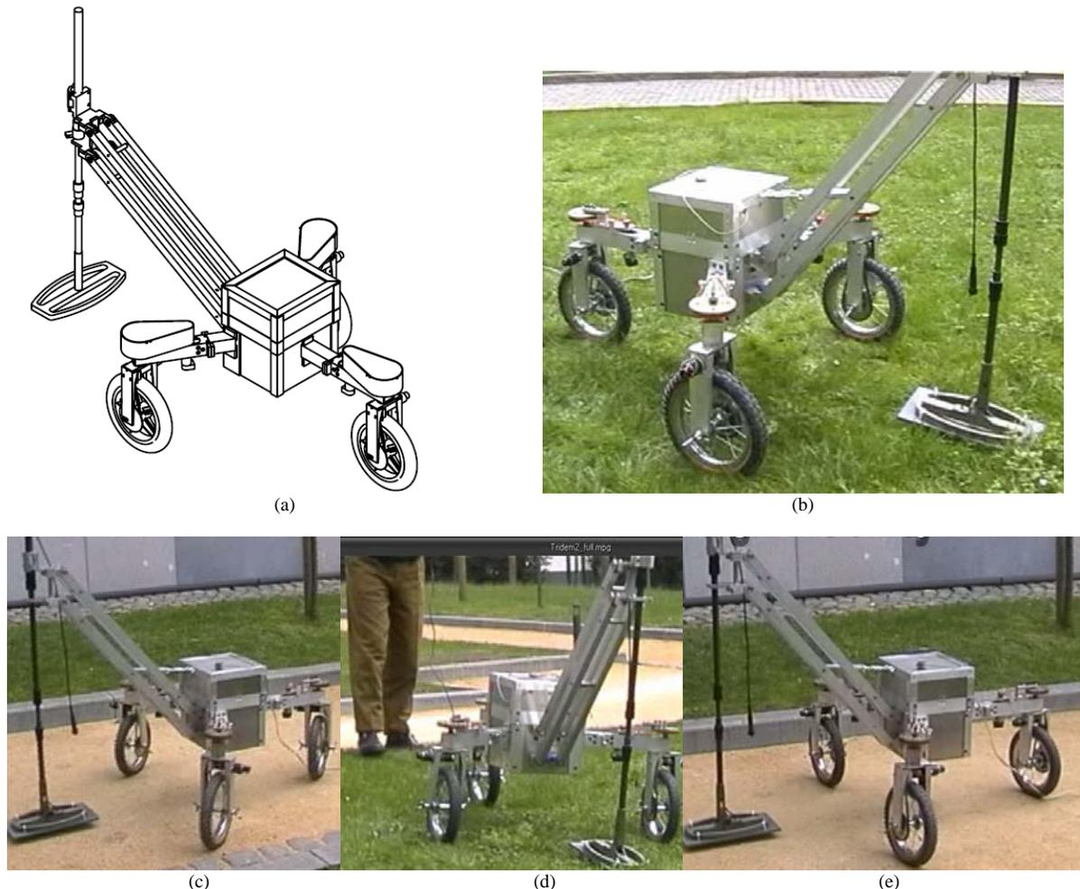
Fig. 4. TriDem wheeled robot: a) 3D design; b-e) real pictures during tests.
