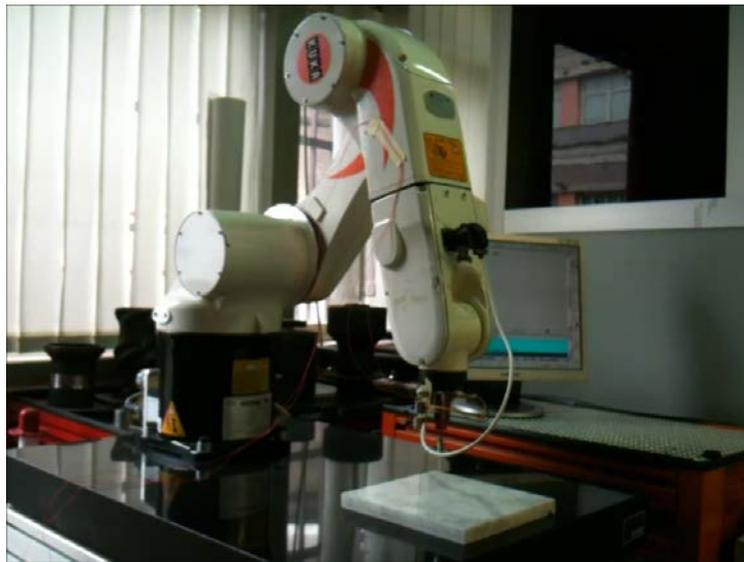
Figure 2. Manipulator with prodder.
