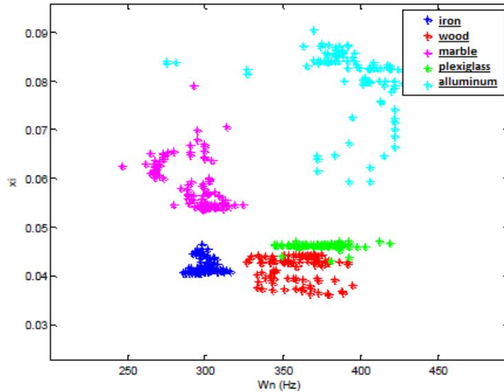
Figure 5. Preliminary classification results Amplitude/frequency for different materials.
