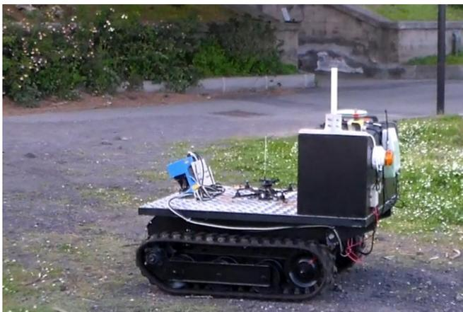
Fig. 5. The adopted UGV platform with the quadcopter on-board ready to take-off.
