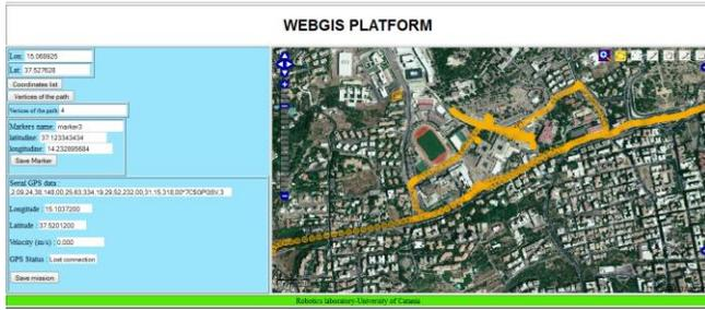
Fig. 4. WebGIS platform developed with the free JavaScript library OpenLayers. On the left side, a large map area, latitude/longitude of the possible paths digitalized, and a mask control for the GPS receiver, are available. On the right side, a retractable layer tree is displayed together with different tools at the top bar.
