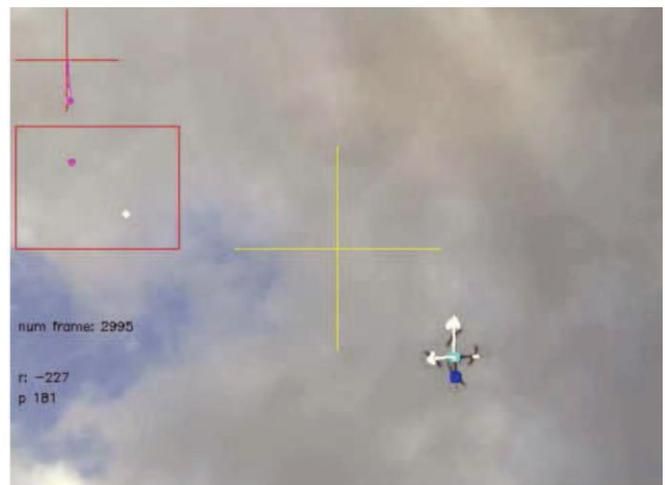
Fig. 6. The vision tracking system computing the position of the quadrotor.
