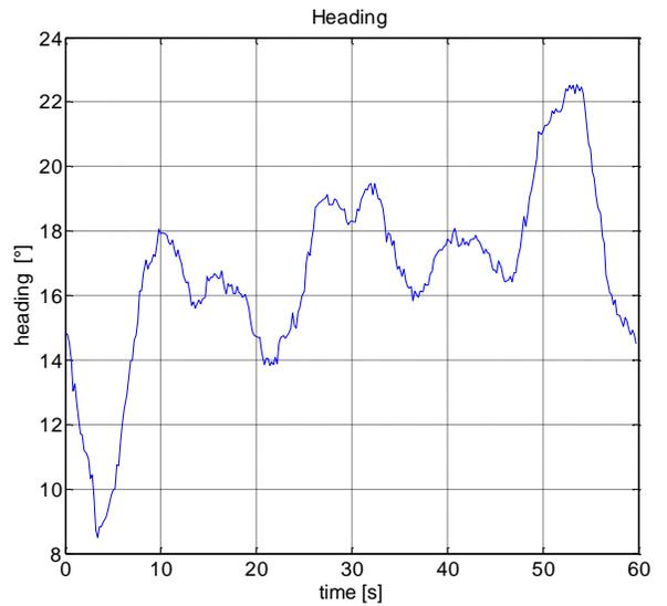
Fig. 10. Heading estimation by means of the vision algorithm.
