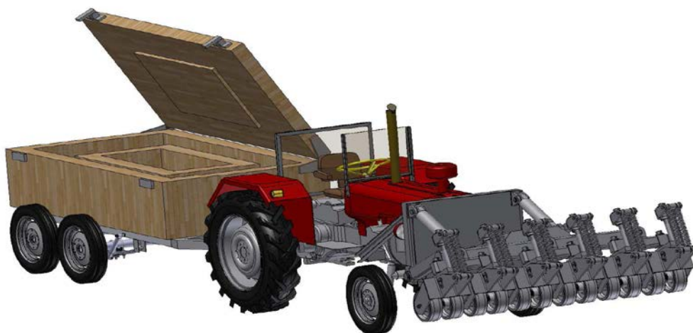
Fig.8. Trailer for temporary storage and transport of explosives with demining machine
