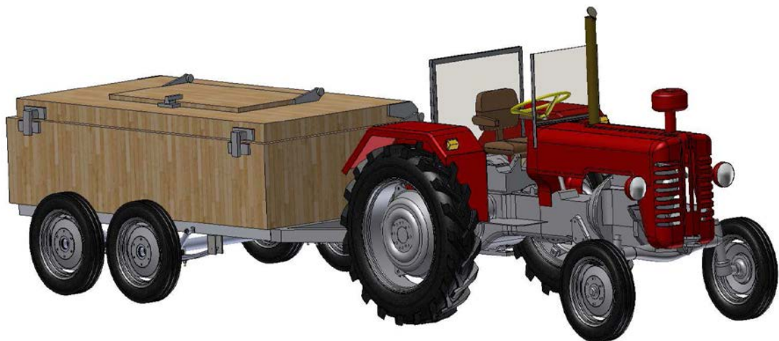
Fig.6. Trailer for temporary storage and transport of explosives and munitions – in closed position
