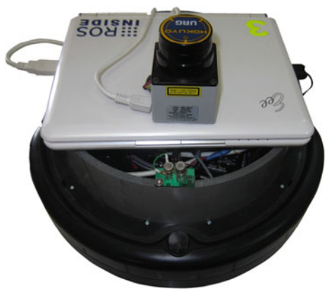
Fig. 20 One of the developed robots containing gas sensors, laser range finder, and iRobot Roomba controlled by a laptop
