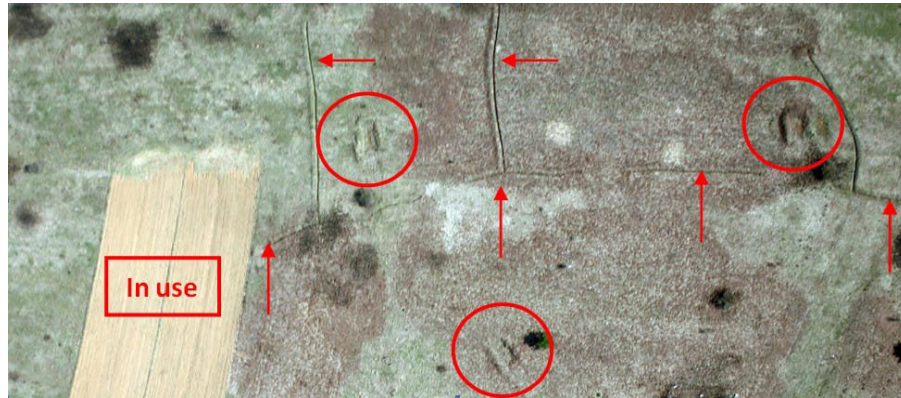
Figure 3. Strong indicators of mine presence (trenches and shelter for heavy weapons) and indicator of mine absence (area in use) within SHA on image of MS3100 camera [Bajic, Krtalic 2009].
