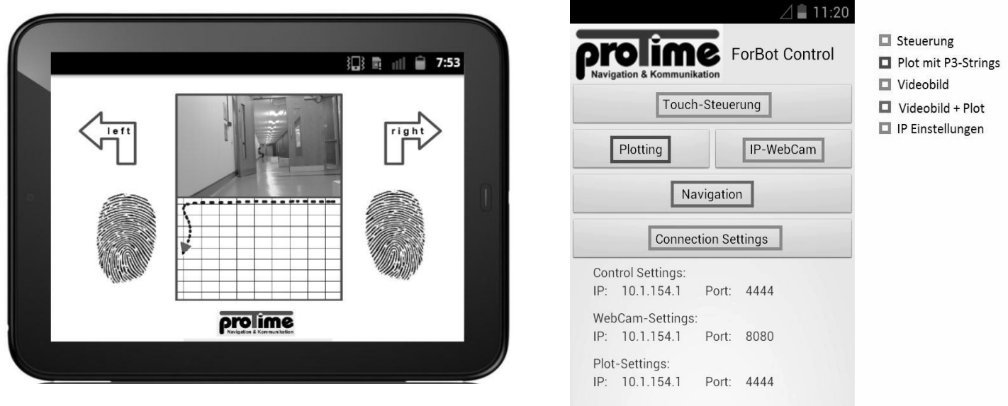
Figure 3: Intuitive GUI of the robot control tablet including video-cam live view and real-time track of robot's relative positions.
