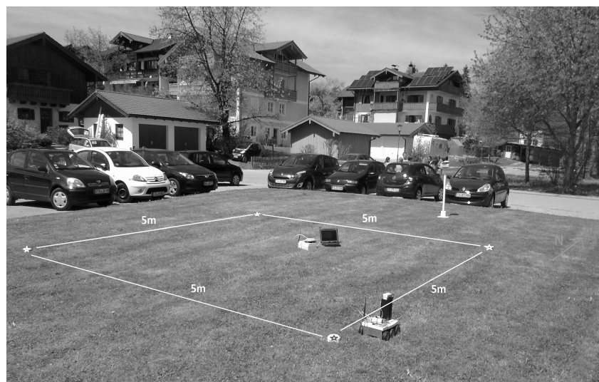
Figure 8: Outdoor test setup for the comparison and combination of IMU- and GNSS-based positioning
