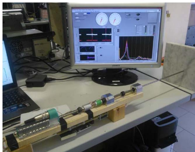
Fig. 5: The experimental setup: the instrumented prodder, a sample of marble and the monitor showing the graphic user interface of the material classification software.
