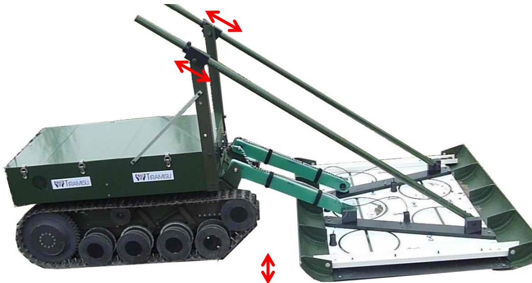
Figure 3 Mounting mechanism with the MCMD and the tEODor platform
