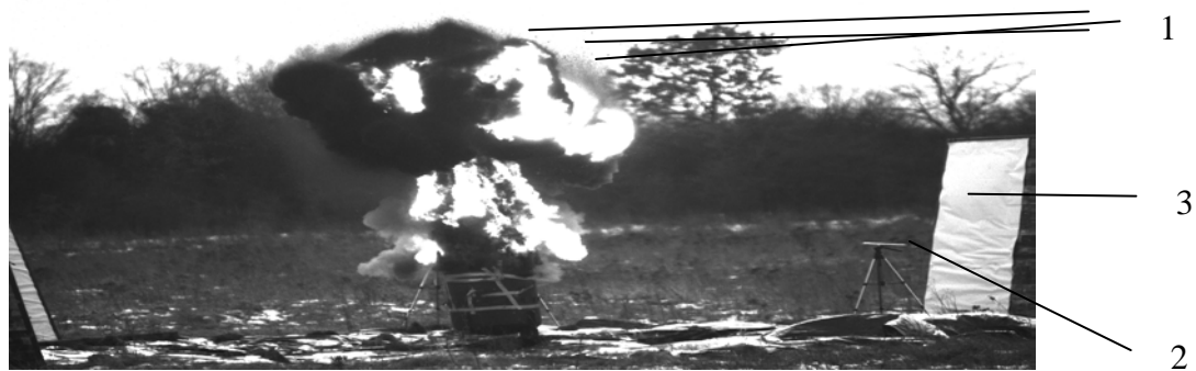
Fig. 3 Effect of detonation of explosive charges in the container 1-steel balls; 2-pressure sensor; 3-control shield
