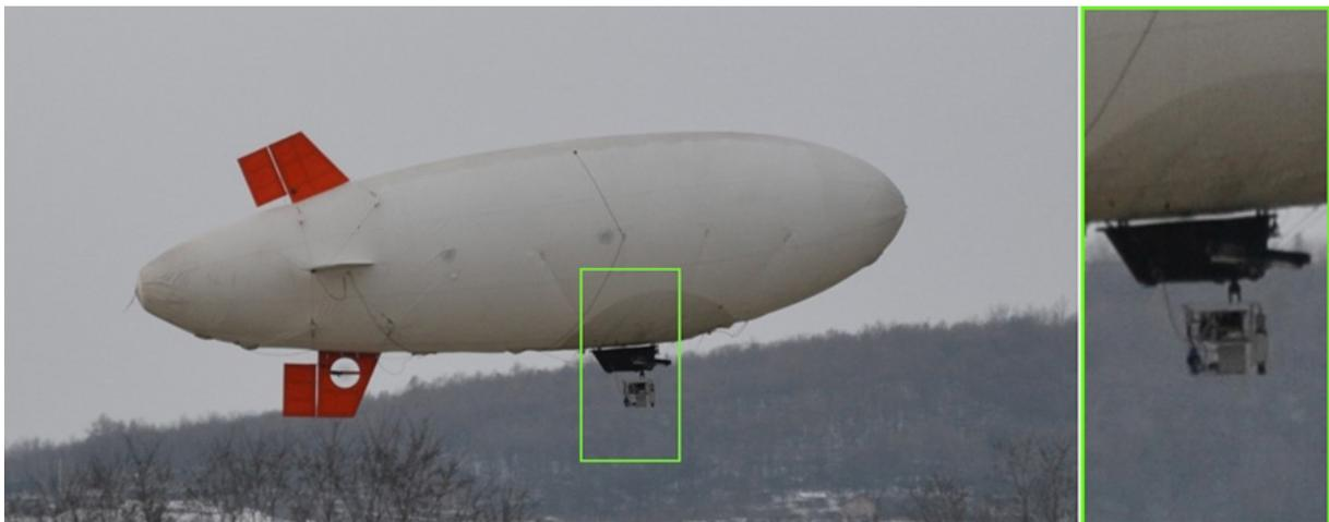
Figure 3. Blimp with T-LHSIS (in two green rectangles).
