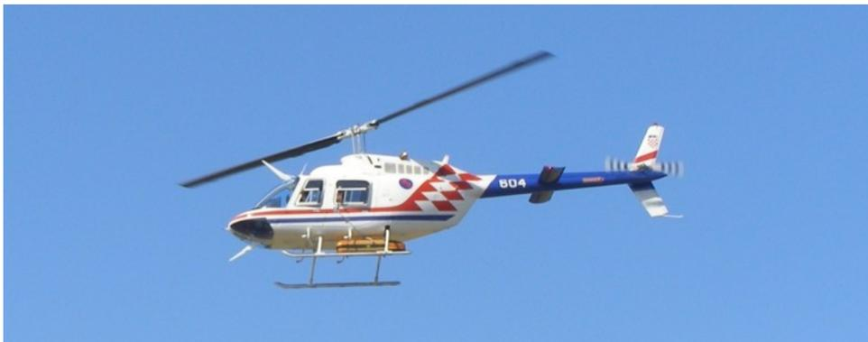
*Figure 4. Helicopter Bell-206 with the T-LHSIS in the orange-black container installed under the helicopter.*
