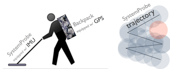
Figure 6: Backpack and Advanced Lightweight detecting system performing coverage of the area to be cleared.
