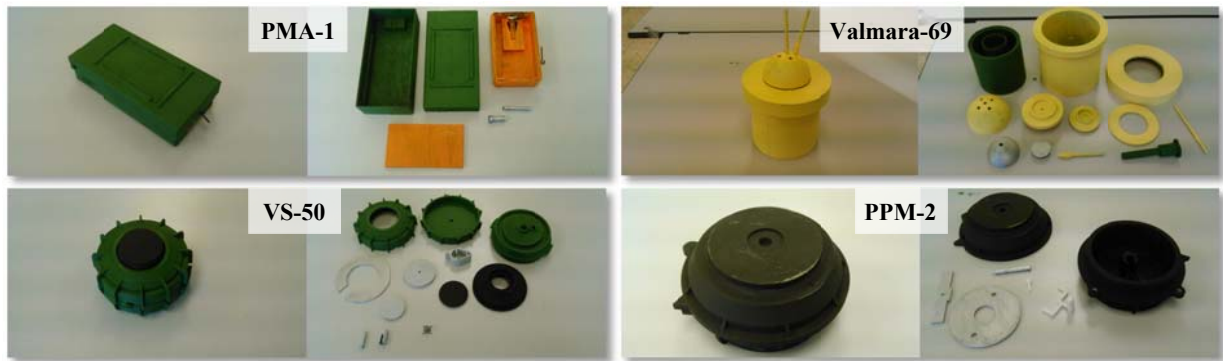
Figure 1. Surrogate antipersonnel landmines designed by CAR CSIC-UPM.
