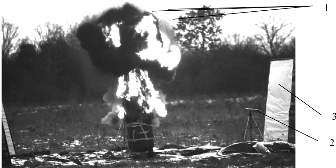
Fig. 9 Effect of detonation of explosive charges in the container 1-steel balls; 2-pressure sensor; 3-control shield
