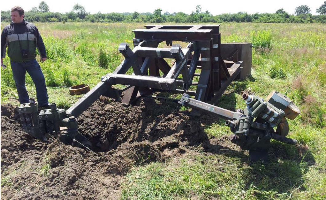
Fig.14 Image mine roller after trial
