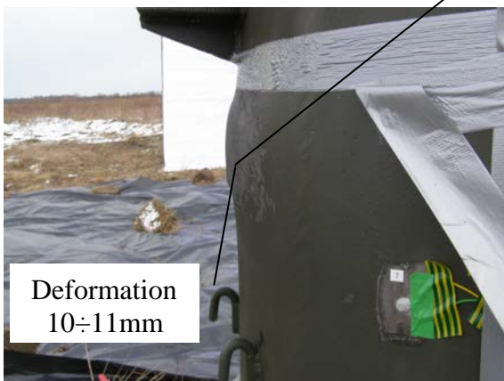
Fig. 10 Deformation of the container side surface-front view (top figure) and side view (bottom figure). The maximum deformation values (Fig. 11) were 10÷11mm and 4÷5mm, respectively.
