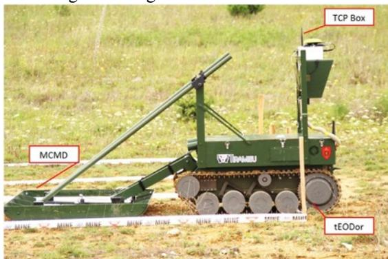
Figure 1 tEODor mobile robot platform with the MCMD and TCP box
