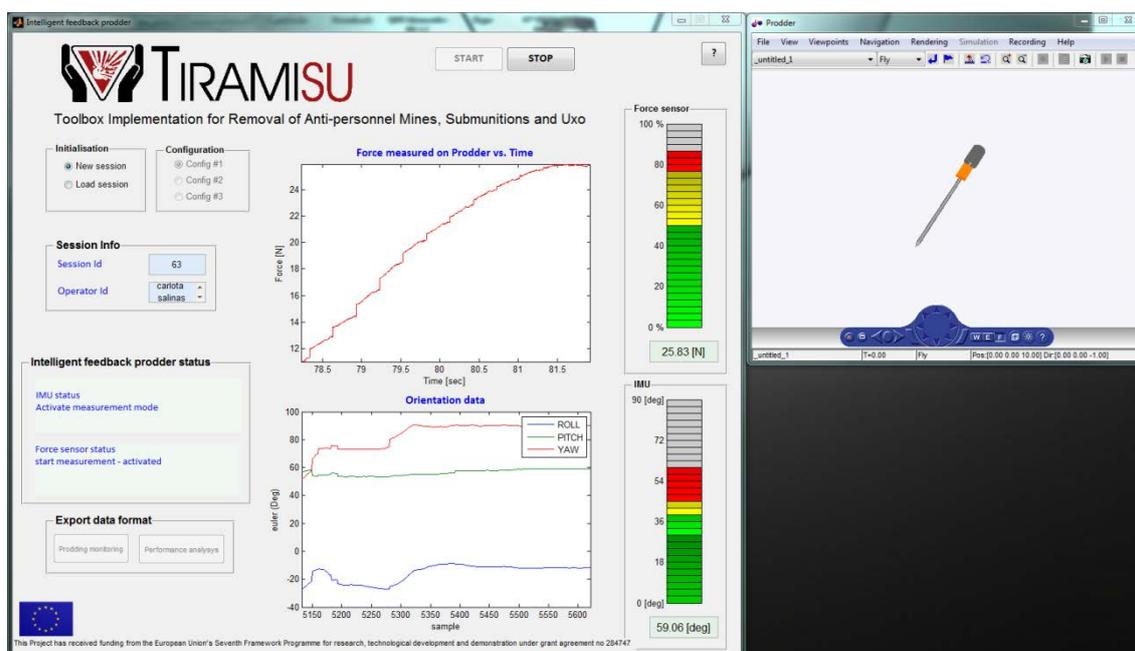
Figure 1. HMI console for the Intelligent Feedback Prodder.
