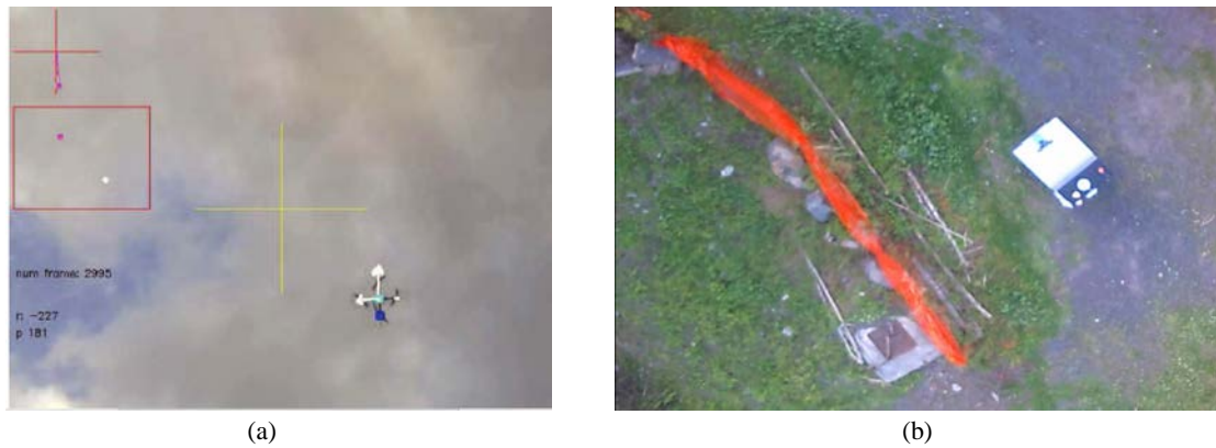
Fig. 4. The vision tracking system computing the position of the quadrotor (left) and the aerial view of the UGV (right).
