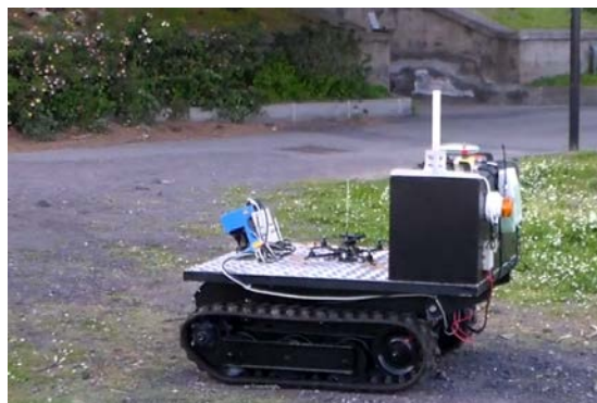
Fig. 3. The adopted UGV platform with the quadcopter on-board ready to take-off.
