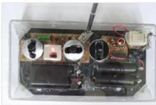
Fig. 7 Remote control system (transmitter and receiver)
