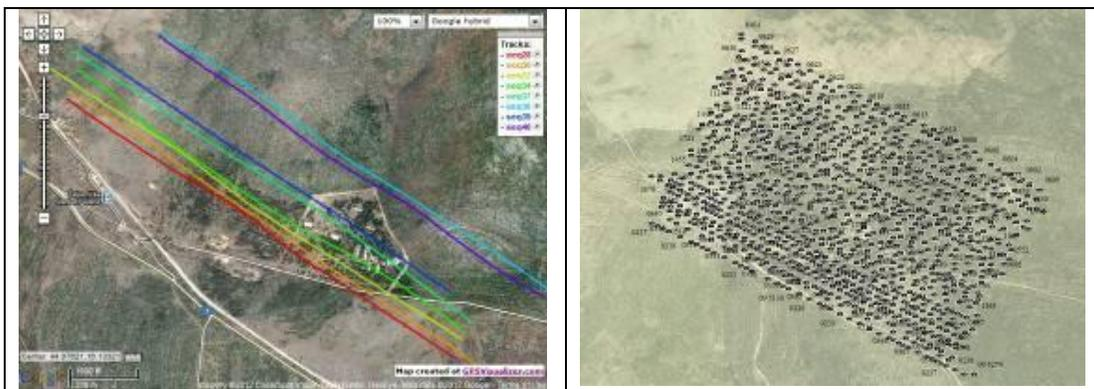
Figure 4. a) Flight routes over the ammunition depot and its vicinity (example). b) Geo tagged positions of the very high resolution airborne images collected by Nikon D90 color camera and MS-4100 multispectral camera. 11-15/06/2012, a TIRAMISU mission CTD and FGUNIZ.
