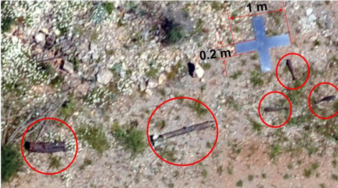
Figure 5. Example of the UXOs and calibration cross on the aerial color image acquired 13/06/2012 in TIRAMISU mission of CTDT and FGUNIZ.
