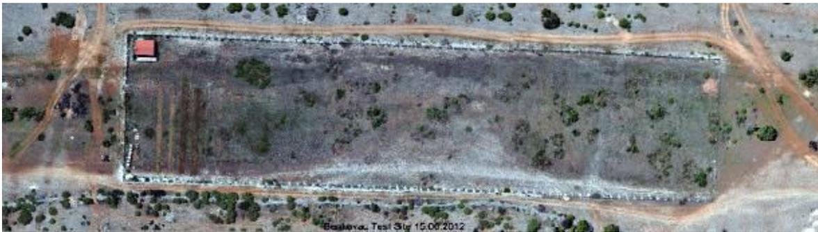
Figure 3. Test site near Benkovac, established 2001., contains 1000 landmines (800 for statistical blind tests). Dimensions 200 x 50 m. Digital ortho photo of the test site Benkovac, derived from airborne images shooting 15/06/2012 in TIRAMISU mission of CTD and FGUNIZ.
