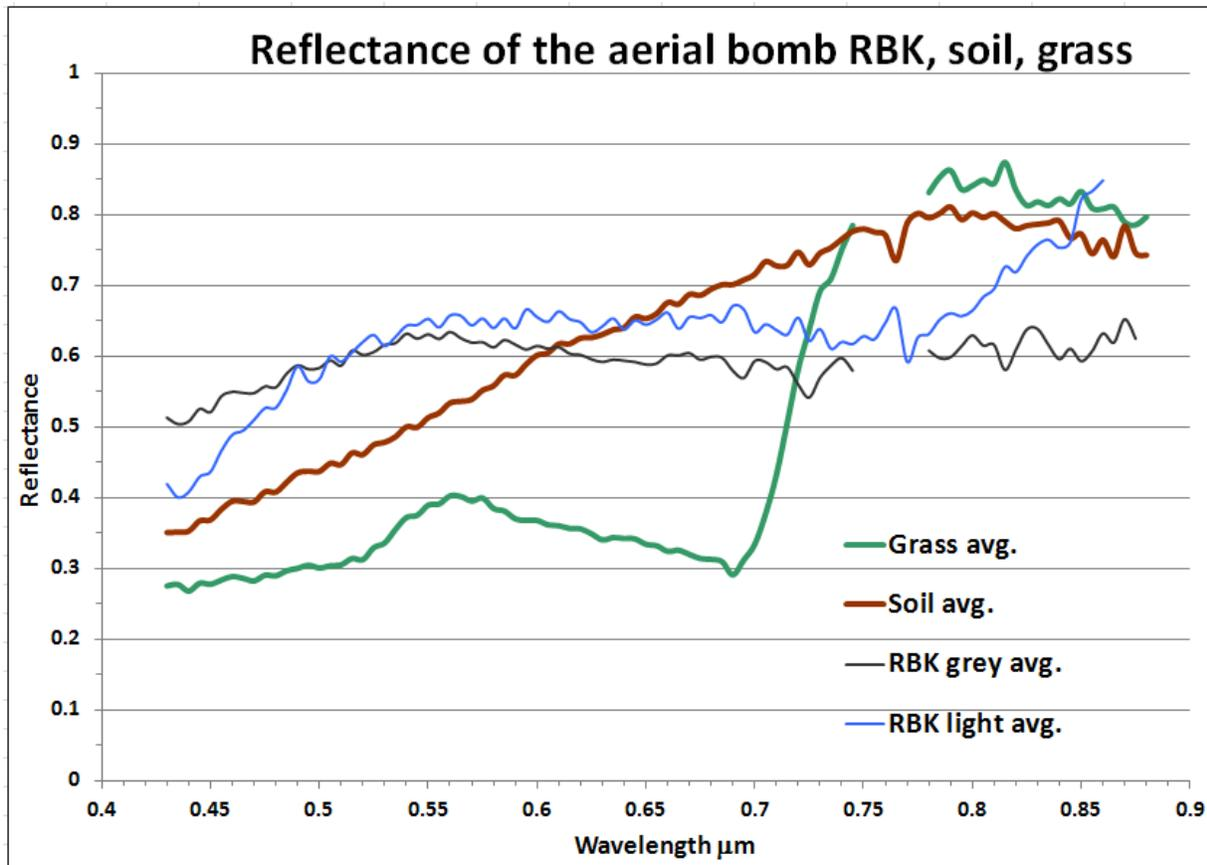
Figure 7. The average (avg.) reflectance of aerial bomb RBK grey, RBK light, soil and grass.
