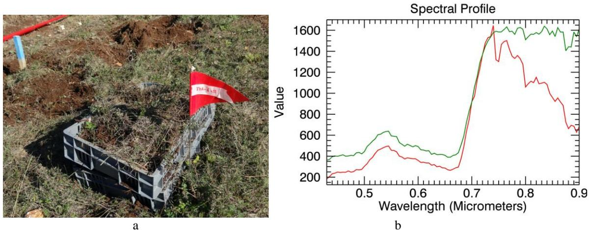
Figure 9. a) Deminer detected, removed the land mine and collected sample of grass which was at top of the mine (TIRAMISU CTD mission, September 2012). Hyper spectral data have been acquired by system shown at Fig. 6a, in a safe area far from the mine field. b) The typical reflectance (green) of the grass collected in the minefield, at top of the land mine, obtained after the atmospheric correction by QUAC (QUick Atmospheric Correction, software ENVI) of the measured radiance (red).
