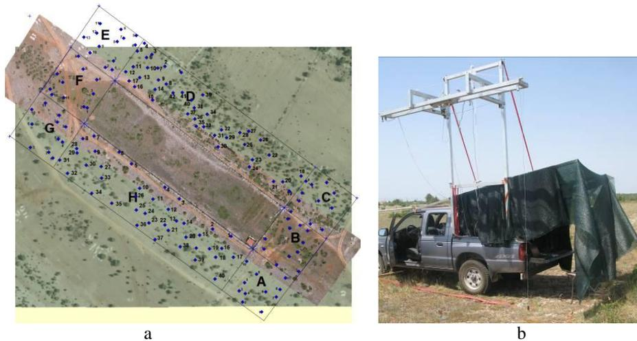
Figure 8. Hyper spectral and bio-chemical sampling the vegetation at test site Benkovac. a) Locations of the random samples of vegetation around the test site Benkovac (July 2012). b) Height of the sensor above the ground level is 3.1 m, enables to cover two squares 1x1 m and the reflectance etalon (LabSphere, Spectralon MS180-1967). The air temperatures in July have been from 30 °C to 40 °C, this caused non smooth carriage movement.
