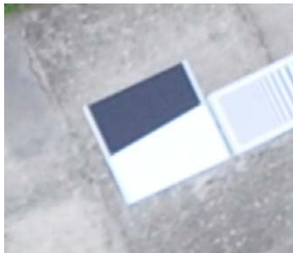
Figure 2. Slant edge target and target with a pair of black and white lines of decreasing width values for MTF.
