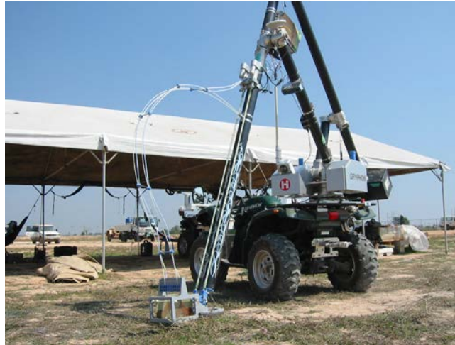
Figure 5. ALIS mounted on a buggy Gryphon (developed by Tokyo Institute Technology). A Vivaldi antenna is attached with a metal detector sensor on the robot arm. The buggy mounted ALIS uses a VNA based GPR for the best performance.
