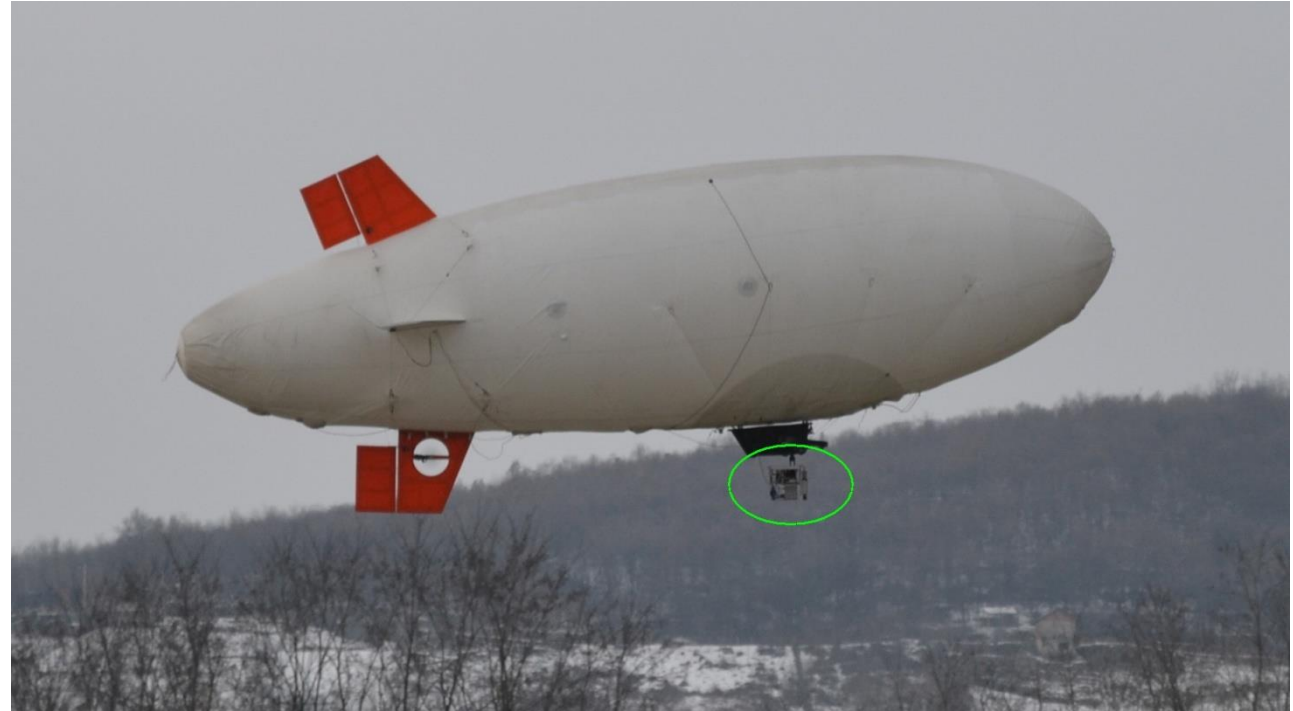
Small system for aerial hyperspectral data acquisition on the blimp (in green ellipse).
