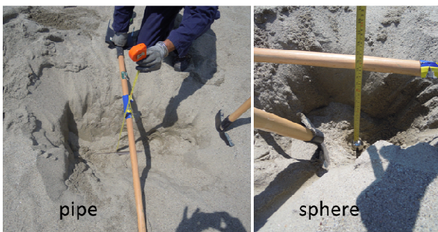
Fig. 10. Example of canonical targets ( \frac{1}{2} " metal pipe and \text{\O}5\text{cm} metal sphere) in homogeneous sandy soil
