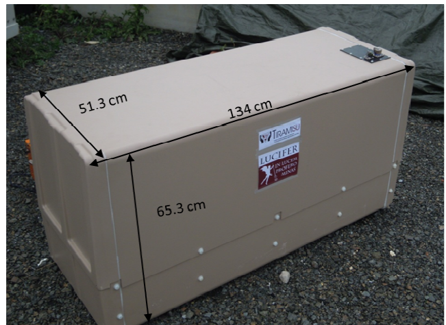
Fig. 8. The new densely-sampled array of air-launched antennas
