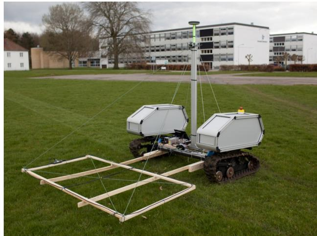
This paper presents the first results from the project. The existing robot platform design has been simplified to lower cost and allow repair in the field with limited tools and spare parts. The robot will be able to utilize various mine detection implements and support different detection methods simultaneously. The FroboMind architecture based on Robot Operating System (ROS) is used for robot control. Software components will be released as open-source for others to build upon.
