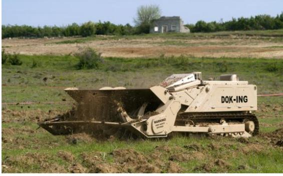
Fig. 1. The MV-4 mine clearance system. Courtesy of DOK-ING company [www.dok-ing.hr](http://www.dok-ing.hr).
