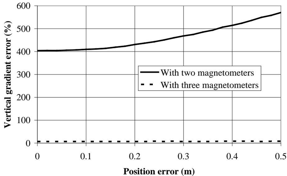
**Figure 2—Vertical gradient errors when estimated with two magnetometers and measured with three magnetometers (10 Hz)**
