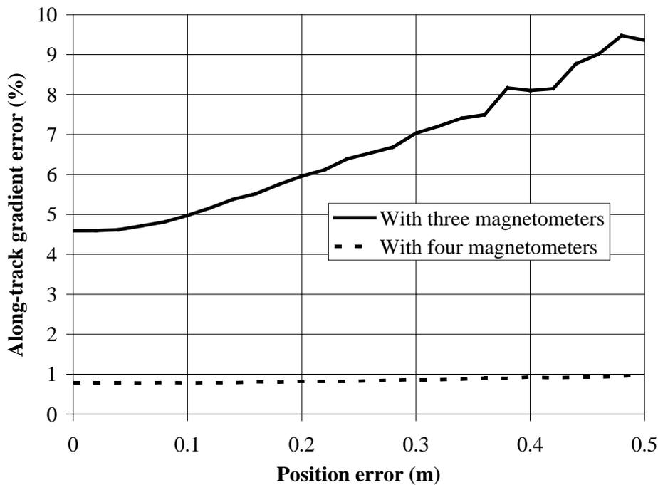
**Figure 3—Along-track gradient errors when estimated with three magnetometers and measured with four magnetometers**
