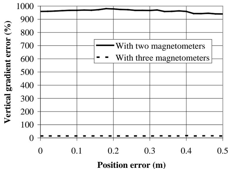
**Figure 1—Vertical gradient errors when estimated with two magnetometers and measured with three magnetometers (1 Hz)**
