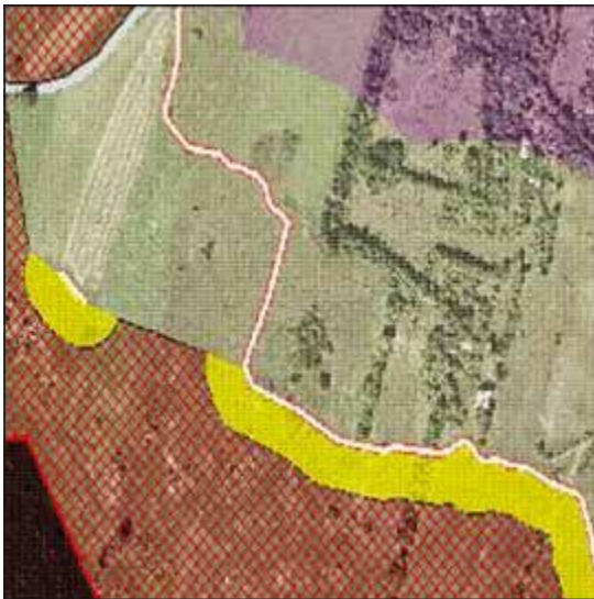
Figure 33. Example of areas and buildings within a defence organization system, which are expected to be free of mines, shown on a DOF2 map. The red line shows a line of forward defence trenches. The line stretches towards North in a function of a hidden road which allows movement of the army to their positions. The yellow area marks the space in front of firing positions which is expected to be free of mines because the positions had to be safe from explosions of their own mines. The area which is not marked north of the yellow polygon belongs to firing positions and it is expected that it is free of mines (this assumption is confirmed by visible cultivated land.
