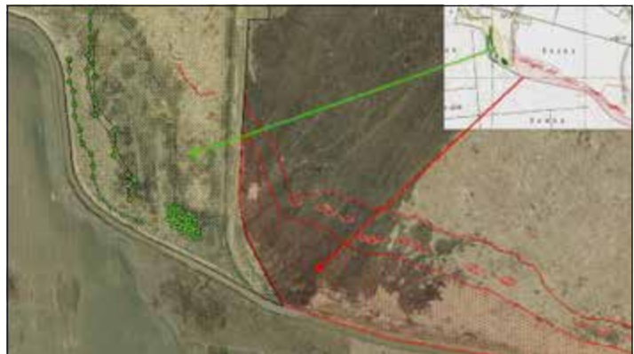
Figure 13. Example of assessment of a new area for demining in line with data about detected mines and fortifications, shown on a 1:25000 scale map (upper right corner of the Figure) and on an orthophoto map, scale 1:2000.
