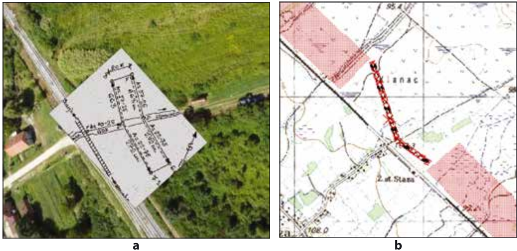
Figure 3. Example of assessment of a minefield belt on the basis of characteristics of a known minefield: a) A sketch of a position of a minefield, from the minefield record, on an airborne colour image. b) Assessment of a barrier minefield belt (irregular polygon in the middle of the Figure) on the basis of data from the minefield record, on a 1:25000 scale map.
