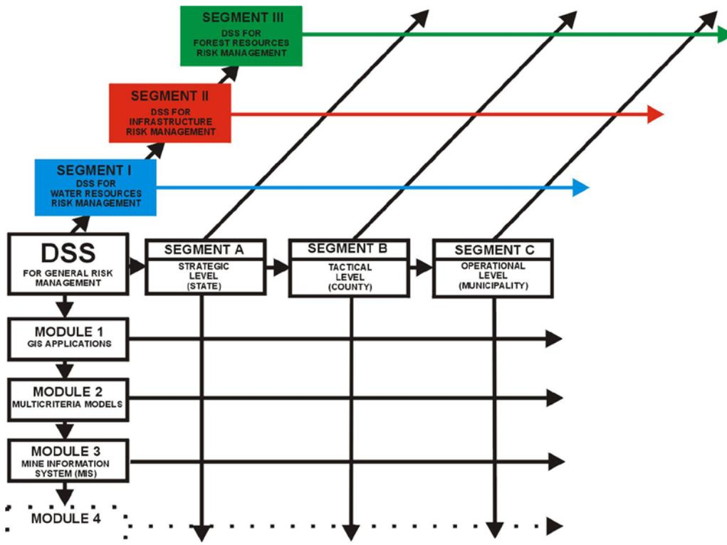
Figure 2: Structural layout of DSS for humanitarian demining operations (Knezic&Mladineo, 2006)
