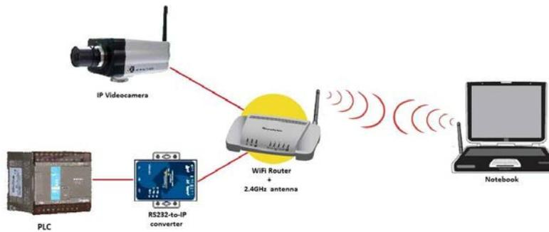
**Fig.5.** Communication module architecture
