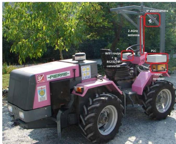
**Fig.6.** PIERRE P796V tractor with hardware installed onboard
