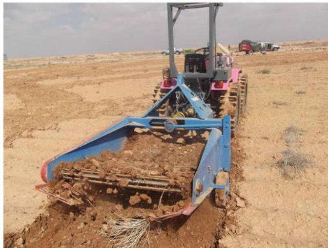
**Fig.3.** LOCOSTRA machine equipped with COTS ground processing tool (produced by F.lli Spedo).
