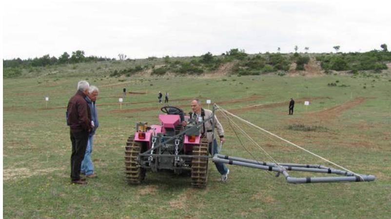
**Fig.4.** LOCOSTRA machine equipped with COTS large loop detector (produced by Ebinger).
