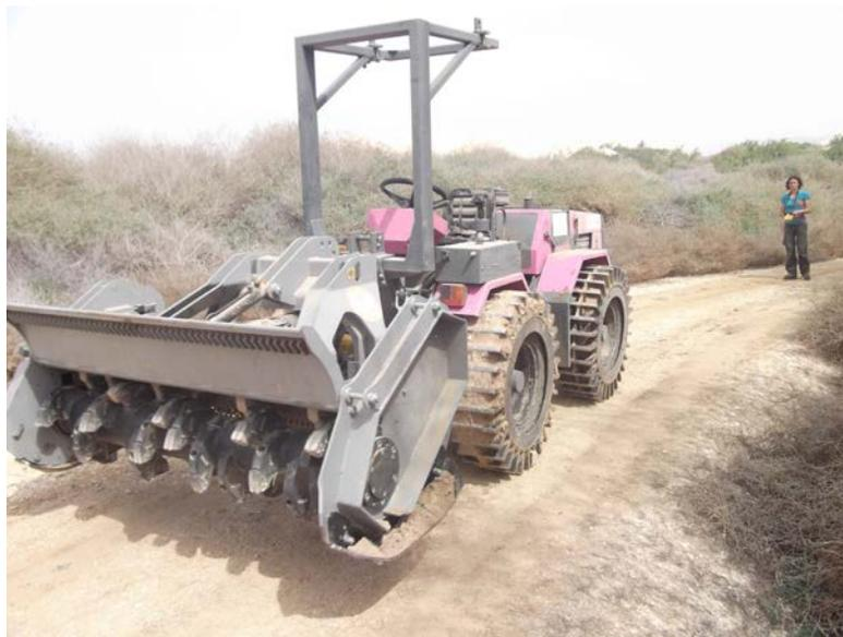
**Fig.2.** LOCOSTRA machine equipped with COTS mulcher (produced by FAE – Advanced Shredding Technologies).
